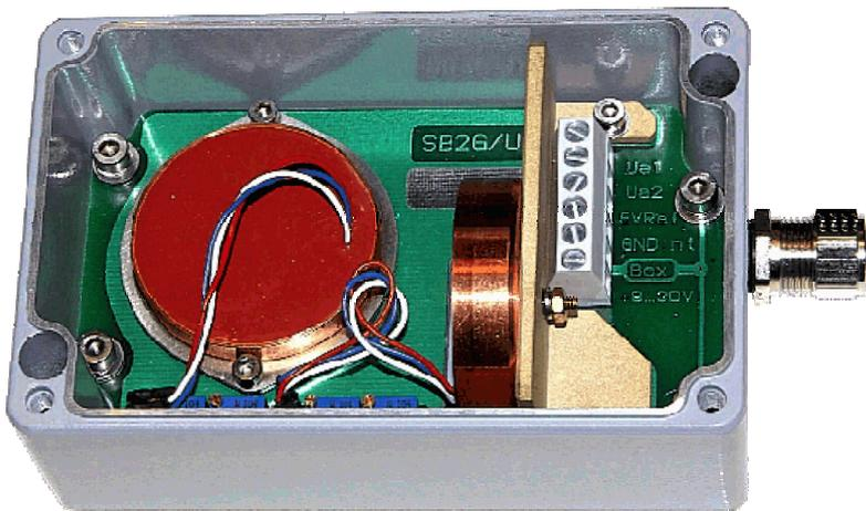
**Sensor box containing two NG inclinometers and two signal conditioners with 0...5V outputs and extensive temperature drift compensation**
